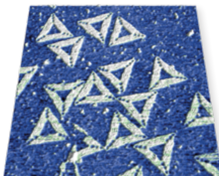
DNA origami triangles , imaged in fluid, 600 nm scan. Sample courtesy of P. Rothemund, California Institute of Technology.
