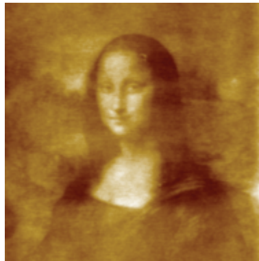
Nanolithography example created by anodic oxidation on silicon, 20 μm scan.
