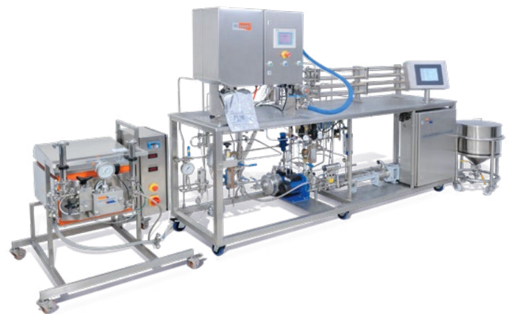
FT94X with homogenisation and true aseptic bag in box packing miniature process line
